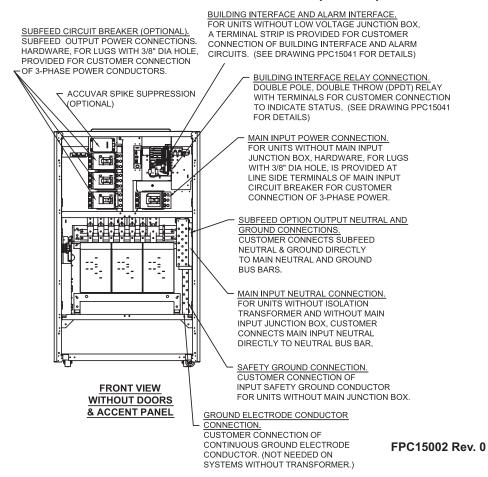
Figure 9 Electrical connection location for 47" cabinet with SqD I-Line panelboard—Rear view
